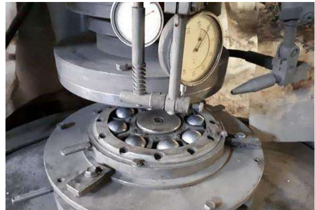
Figure 2 – The location of ceramic balls in the device on the ball-grinding machine VS-D204M
