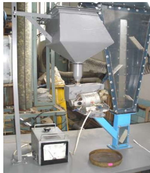
Figure 2 — Assembled representation of the laboratory unit for pneumatic classification [7]
