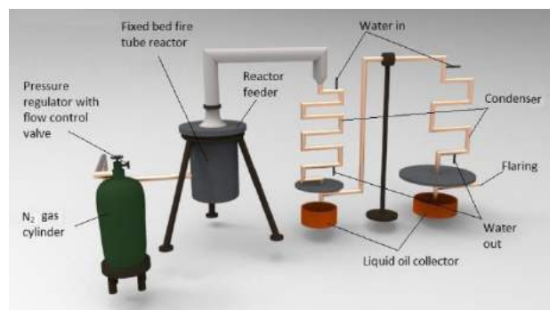
Figure 2 – Schematic diagram of a fixed bed pyrolysis plant
