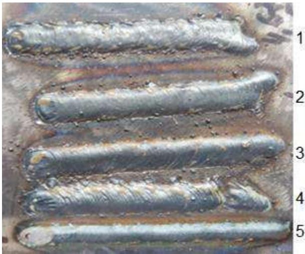
Figure 4 – Weld beads for the different frequencies: 1 – 4.5 Hz; 2 – 4.0 Hz; 3 – 3.0 Hz, and 4 – 2.5 Hz; 5 – without oscillations
